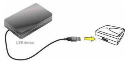
3.4 Connect the Network USB over Network Server to the router or switch/HUB with the Ethernet cable.
