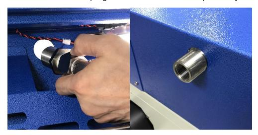
Insert the flat washer to bulkhead coupling.
