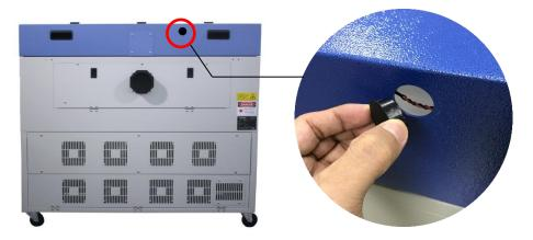
Release the hex nut and flat washer from the side of the bulkhead female coupling.
