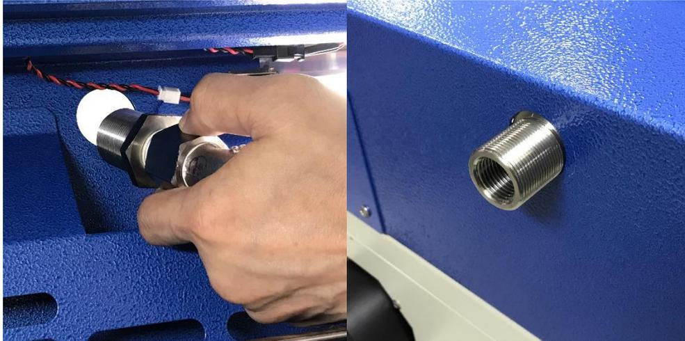
Insert the flat washer to bulkhead coupling.
