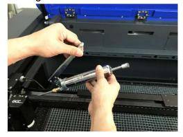
6. Seal the lubrication slot plate back to the X rail
