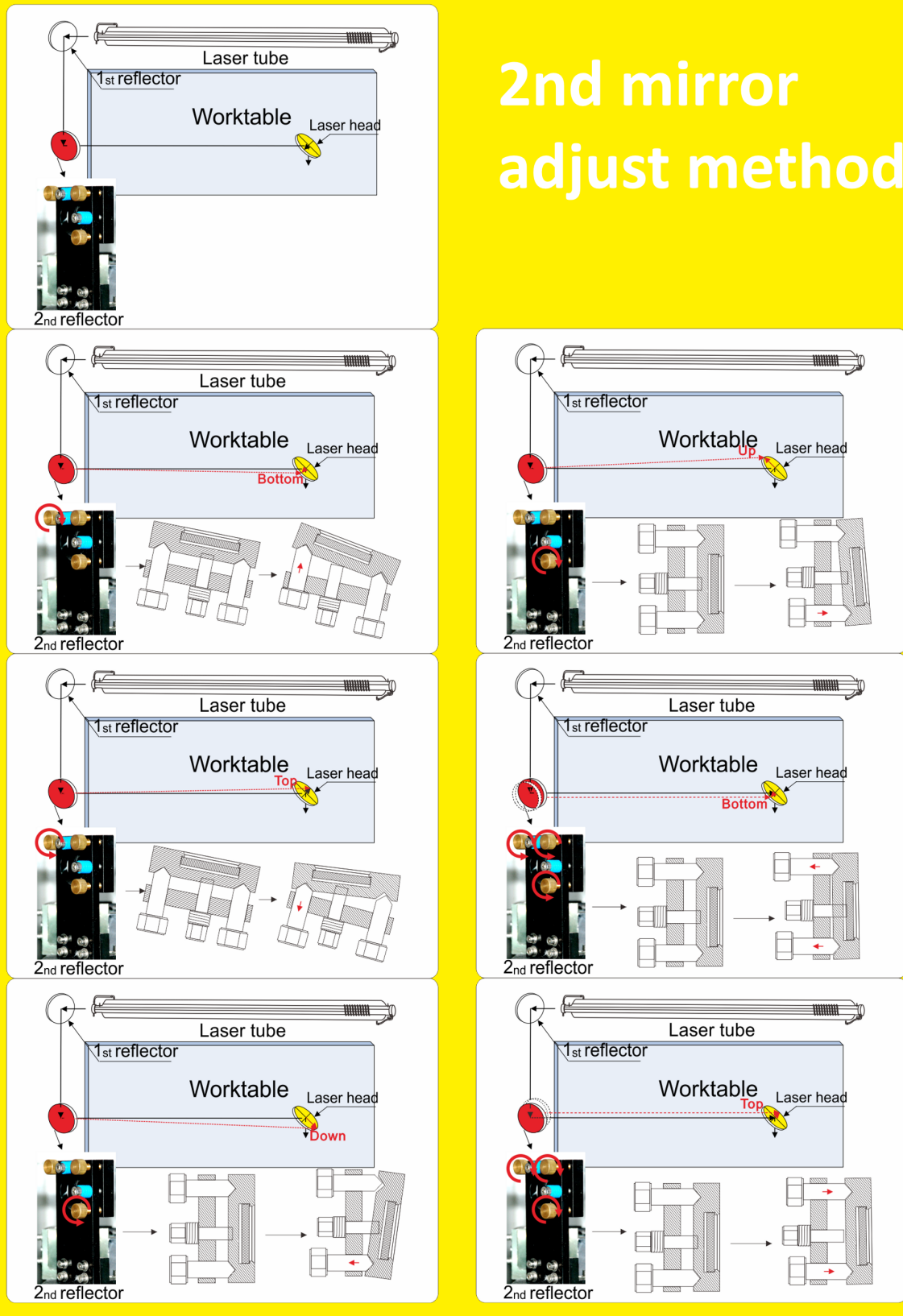
Figure 2-4: 2nd mirror adjust method
