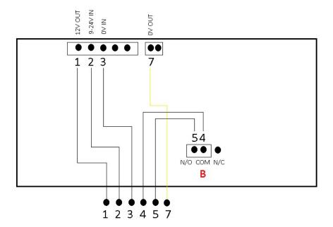
FILTER CONDITION ALARM (Changeable between N/O and N/C in the setup menu)
